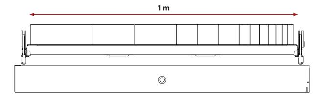
The storage capacity for each drawer is 5 meters of linear tools, which can be both Promecam and W-Style, for a maximum load of 350kg each.
